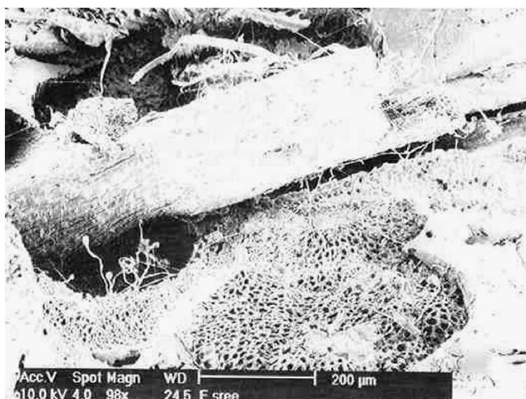
Figure 19. SEM of impact fracture of gamma irradiated, acetylated oil palm fiber/PF composite ( \times 98 ).
